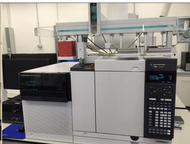
GC-MS triplo quadrupolo Agilent 7010
